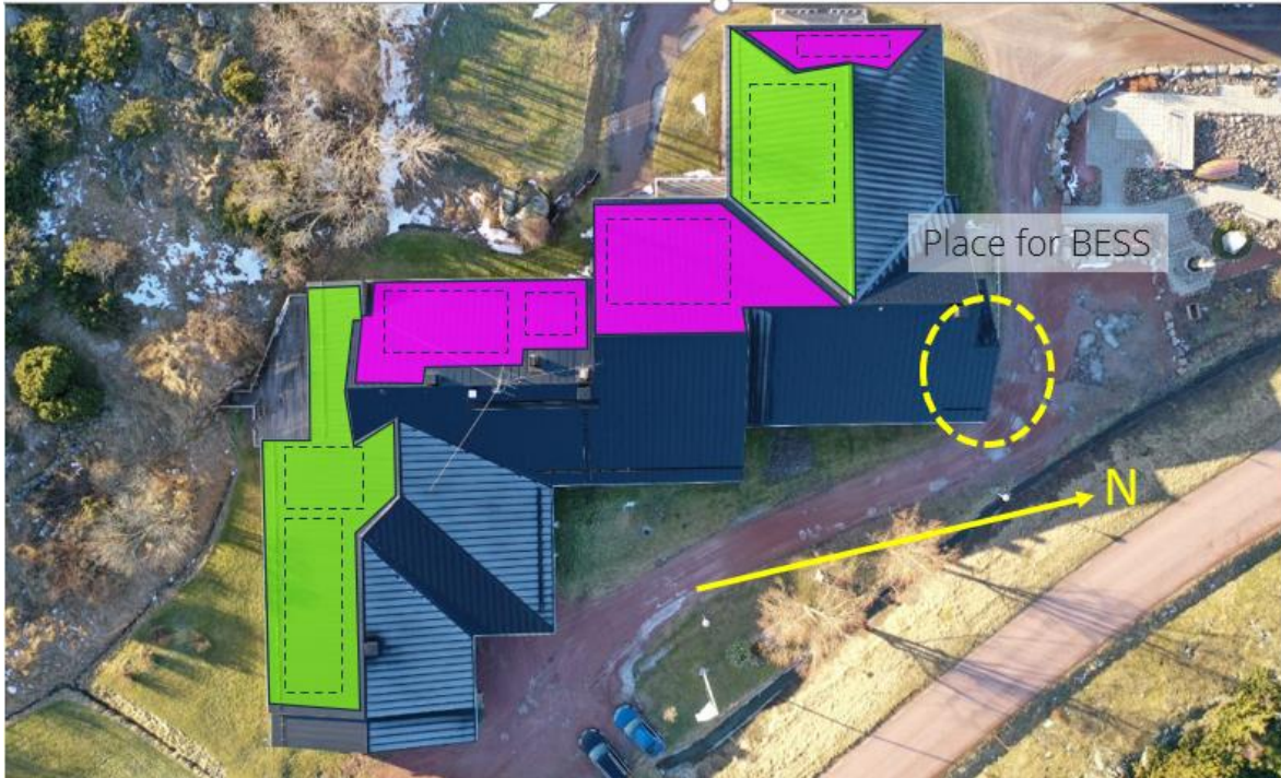
Figure 3: Satellite image of the nursing home with PV arrays and BESS location indicated
